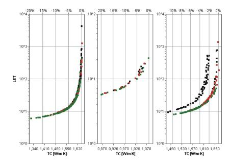
The Single Measurement Plot In addition to the optimal interval, thermal conductivity values are calculated from all intervals having a minimum LET value. For checking sample preparation and measuring conditions, the Single Measurement Plot displays the LET values of all
